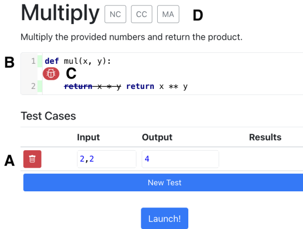
Fig. 1. The MUTTLE interface. Each exercise lets the user create, modify or delete test cases (A). If their test cases pass, they are given BRANCHCOV feedback in the colored gutter next to the line numbers (B) or MUTATIONCOV feedback in the form of bug badges above the lines of code where mutations were made (C) In this example, the statement return x * y was mutated to return x ** y . The interviewer used the toggles at the top of the screen to switch between no coverage, code coverage, or mutation analysis feedback, based on the experimental condition (D).
