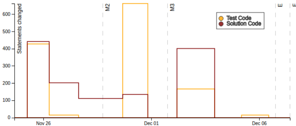
Figure 4.8: An example of a project with an intermediate metric score for test writing, with room for improvement. Notice the irregular bursts of test code writing, and that work started after the first Milestone was due. This project was in the 64th percentile for Incremental Test Writing, and in the 69th percentile for the Early/Often Index.
